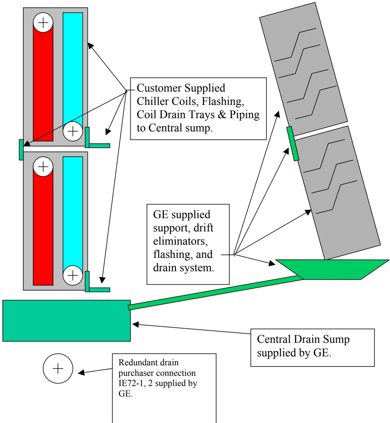
Figure 3: Chiller Coils and Drift Eliminator Scope of Supply.
