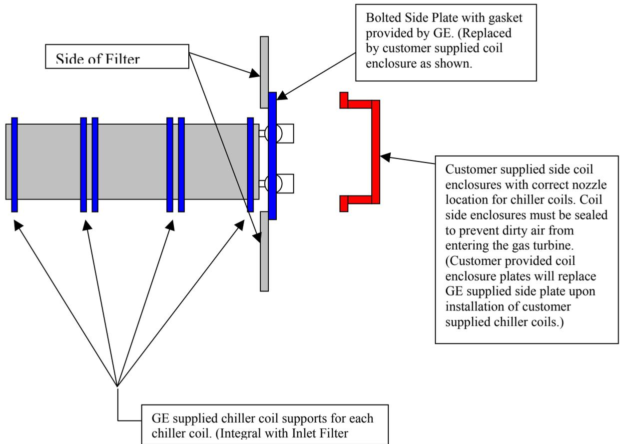
Figure 1: Maximum Chiller Coil Dimensions and Supplied Equipment.
