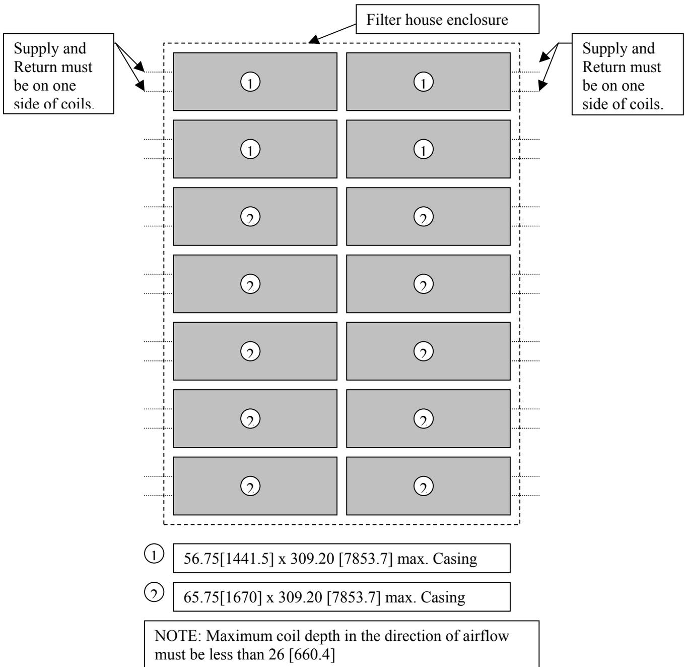
Figure 2: Chiller Coil Arrangement.
